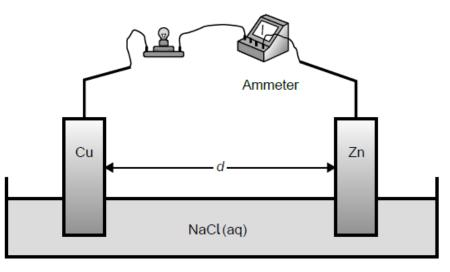
The student gradually increased the distance, *d*, between the electrodes to study the effect on the initial current, *I*, passing through the light bulb. The student hypothesized that the initial current would be inversely proportional to the distance between the electrodes.
